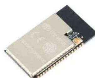
Figure 7. Wifi module Esp32
