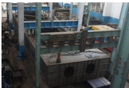
Fig 2. Photograph of the loading arrangement of the experimental model
